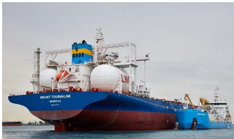
LNG Bunkering of World's first Newcastlemax Bulk Carrier
